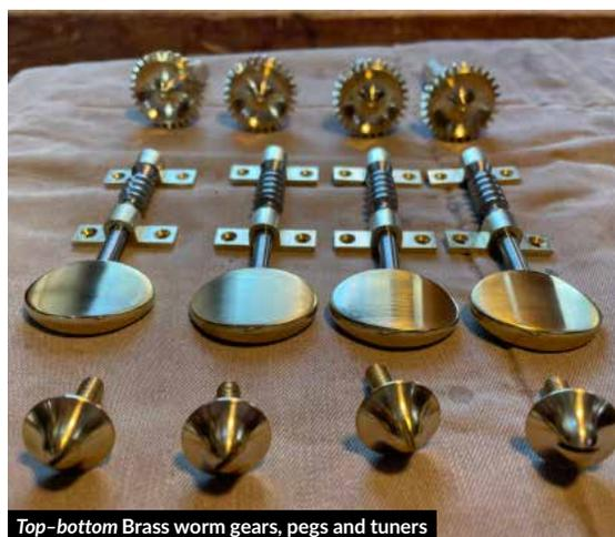
Top-bottom Brass worm gears, pegs and tuners
