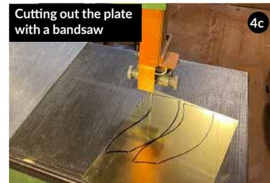
Cutting out the plate with a bandsaw
