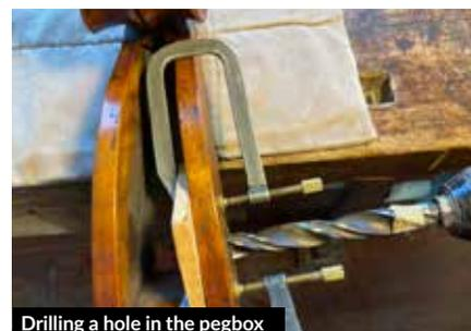
Drilling a hole in the pegbox
