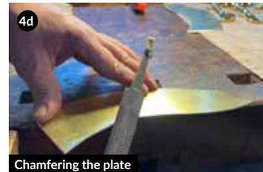
Chamfering the plate
