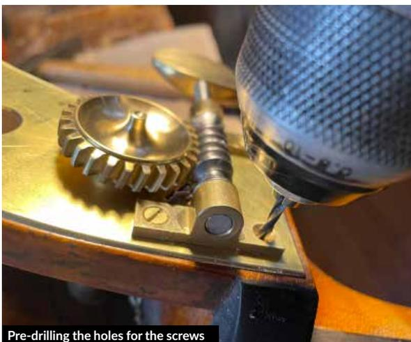
Pre-drilling the holes for the screws
